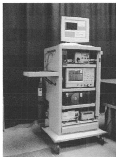
FIG. 1. (a) Schematic diagram illustrating the modular tr-LIFS apparatus setup; and (b) photograph of the system hosted in a mobile endoscopic cart; PMT: multichannel plate photomultiplier tube; ICCD: intensified charge-coupled-device camera.
